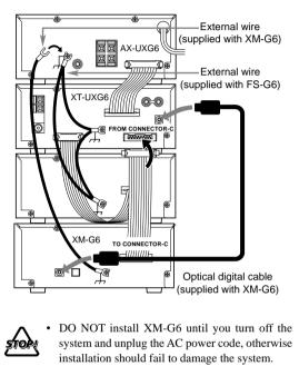
• DO NOT change the vertical stacking order of XM-G6 as illustrated to avoid heat buildup.
